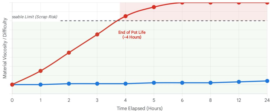
Comparison of effective processing windows. Platinum systems (top) exhibit rapid viscosity build-up after mixing, necessitating immediate use. M-Cor Peroxide systems (bottom) remain stable at ambient temperatures, enabling consistent long-run extrusion without degradation.
