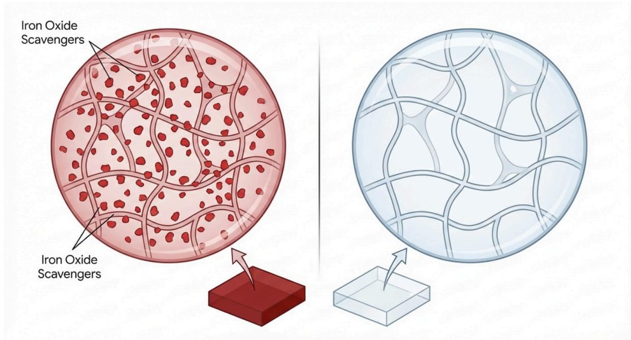
Micro-structural comparison. Left: Standard Peroxide matrix saturated with Iron Oxide particles (Red) for heat stability, blocking light transmission. Right: M-Cor Translucent Peroxide matrix using advanced non-pigmented stabilizers, allowing full optical clarity for inspection.
