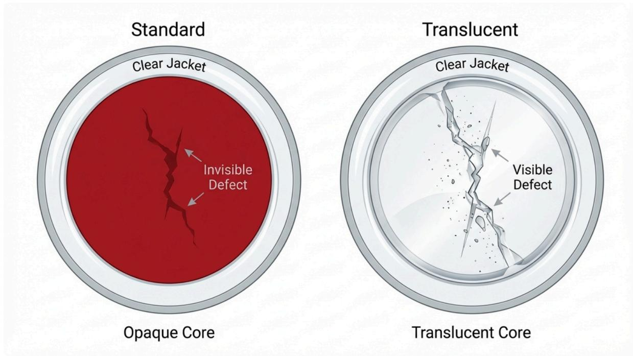
Comparative visibility of core defects. Left: Standard Iron-Oxide Peroxide Core (Red) obscures internal stress fractures and chemical ingress. Right: M-Cor Translucent Peroxide Core reveals internal voids, particulate contamination, and core degradation without disassembly.
